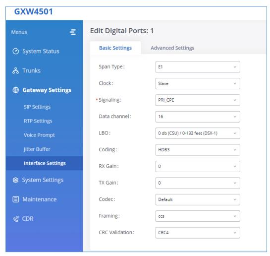
Figure 46: Digital Port Configuration
