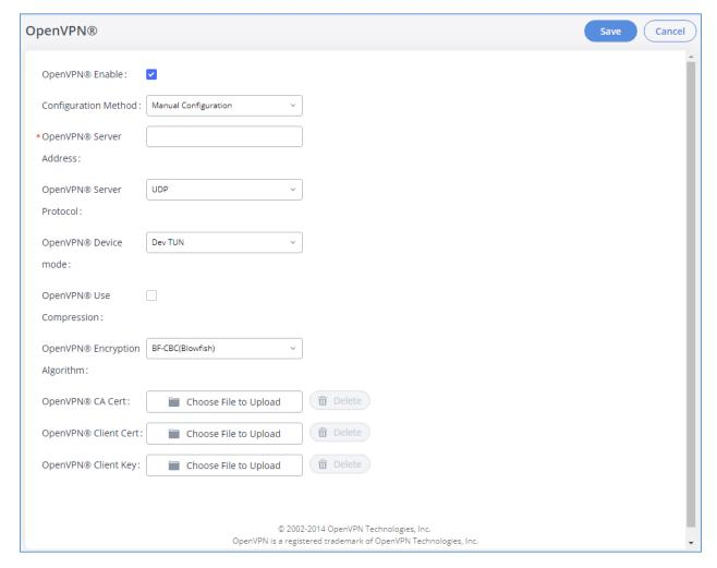
Figure 24: OpenVPN® Feature on the GXW450X
