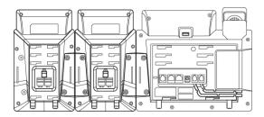
**3.** Connect the Ext jack of the IP phone and the Ext in jack of the expansion module using one supplied cord.
