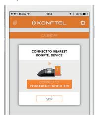
The device name displayed is the name shown on the screen of that Konftel 300IPx phone. (This text can be altered. See SCREEN and text settings in the administration manual for the Konftel 300IPx).
