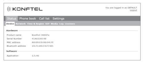
You can find the phone's serial number, network port address, Bluetooth address and current software version on the **Basic** tab. Settings made by the administrator for the network, time server, SIP accounts and media are on other tabs.
